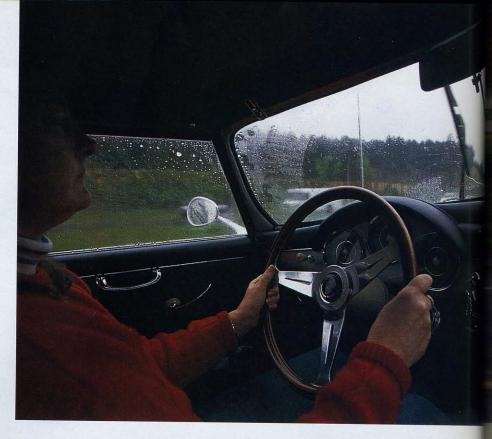
lization, you're free to rediscover how much fun operating such a lithe package can really be. Steering is perfectly weighted and informative through the 15-inch wide Derrington wood wheel. Driving a sports car without power assist is a rare treat these days, and the lack of boost means you're not depending on a slave unit to interpret what's transpiring at the front contact patches. The front suspension geometry is also revised to increase caster angle for better response.
